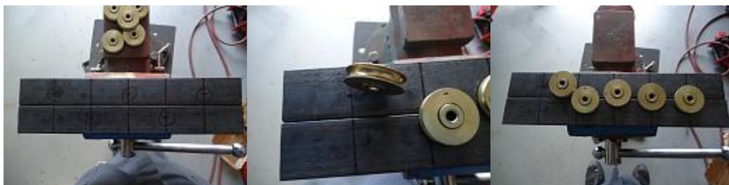
After you have the rollers spaced out and layed out correctly center punch the roller holes and drill the holes.
